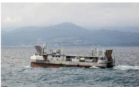
The overall design incorporates four ramps, with the two hulls tied to liaison arms and a moving platform, that is raised by hydraulic jacks. CMR is accustomed to this level of complexity when **integrating systems** to perform a variety of local or remote tasks.
